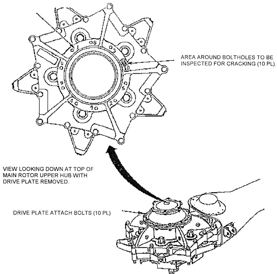
**Figure 1. Main Rotor Upper Hub Assembly Inspection**
