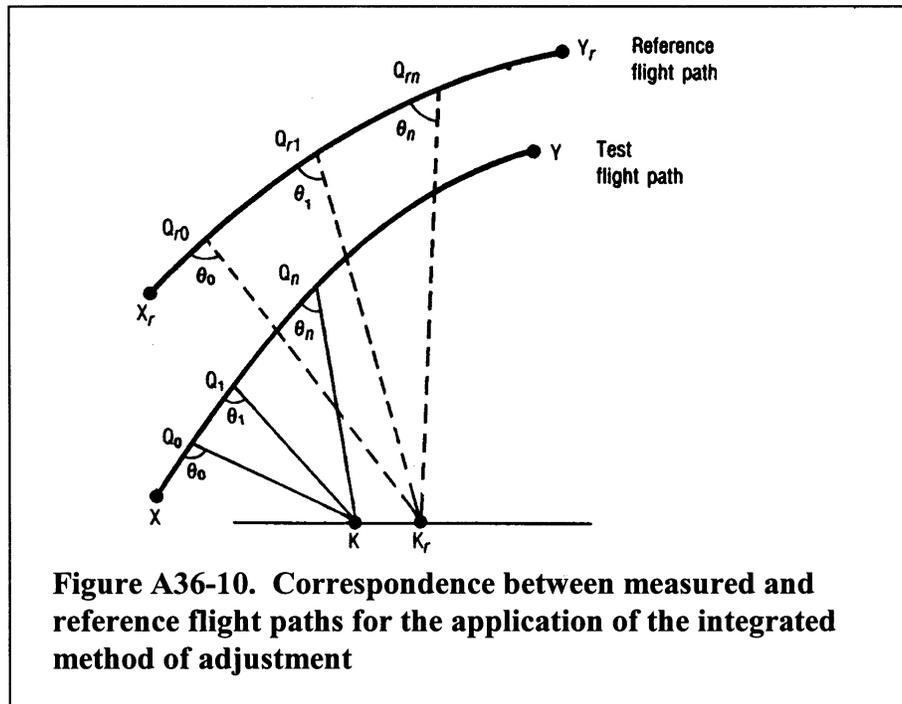
**Figure A36-10. Correspondence between measured and reference flight paths for the application of the integrated method of adjustment**
