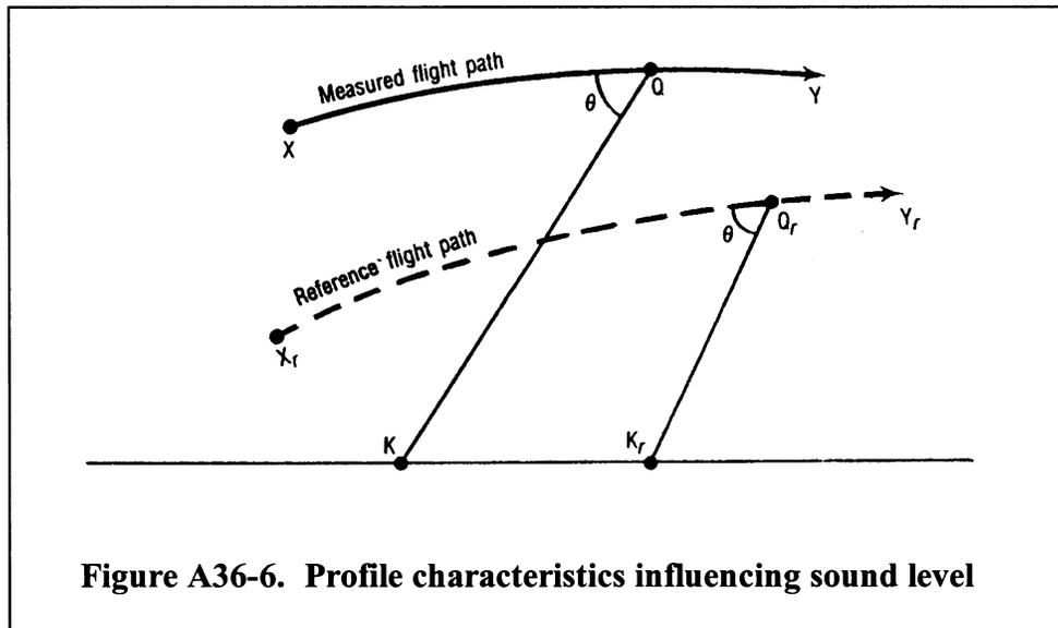
and reference noise propagation paths,  $Q_r$  being determined from the assumption that  $QK$  and  $Q_r K_r$  form the same angle with their respective flight paths.
