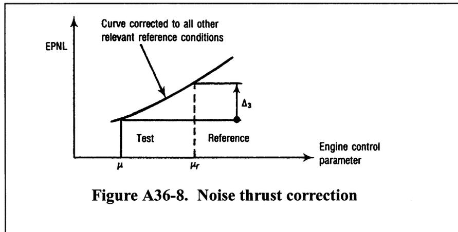
Figure A36-8. Noise thrust correction
